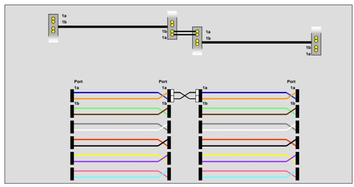
Figure 3: Optical fibre polarity within channels containing fixed cabling with duplex interfaces
