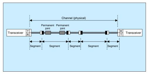
Figure 1 - A duplex transmission channel containing two optical fibres
