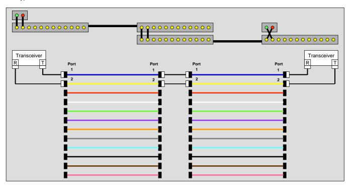
Figure 2: Optical fibre polarity within channels containing fixed cabling with simplex interfaces
