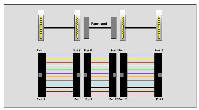
Figure A.1 - Optical fibre polarity within channels containing fixed cabling with array interfaces
